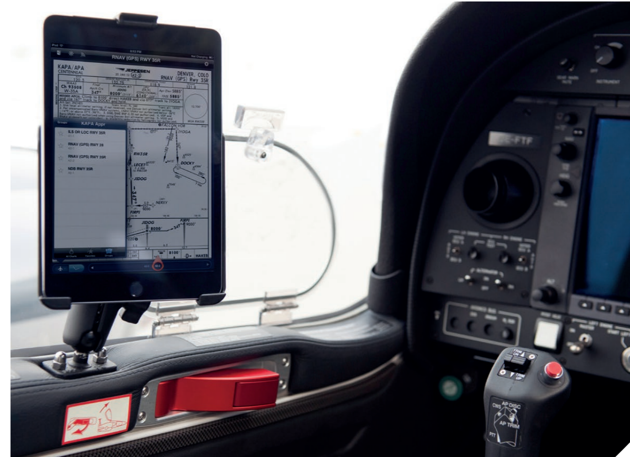
Built-in tablet mount provisions for pilot & co-pilot armrests (tablet and cradle for visual purposes only)
