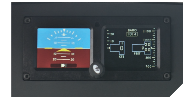
Standby electronics (instead of back-up instruments)
