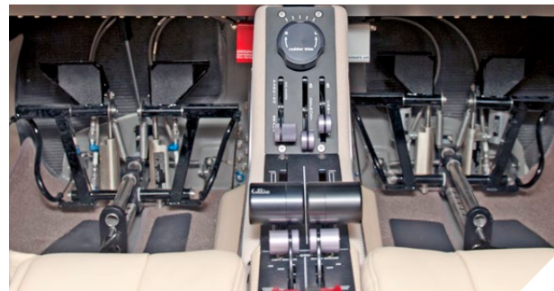
Electrically operated, adjustable rudder pedals for pilot & co-pilot
