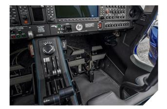
Electrically adjustable rudder pedals for pilot & co-pilot
