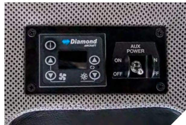
Air conditioning / RACC system (powered by an additional alternator)
