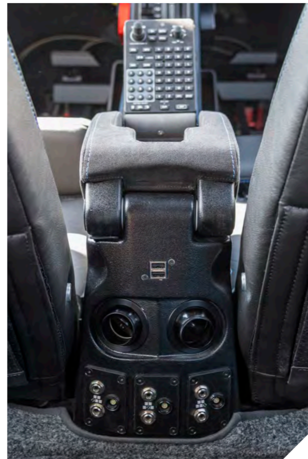
USB power outlets for pilot & co-pilot and passengers in the 2 nd row Dual headset plugs (LEMO connector + standard jack connector)
